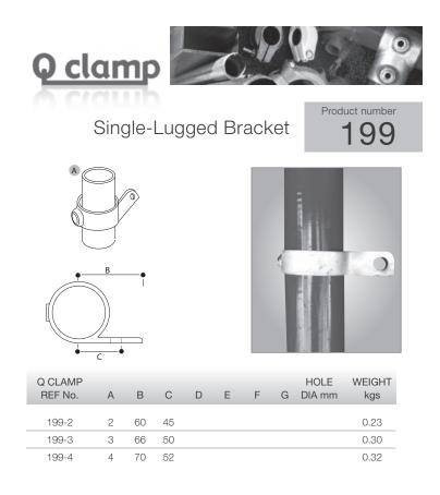
Often used for mounting boards practically flush with tubes. Fixing holes suit a wide range of common mechanical and chemical masonry anchors. The tube cannot be joined within the fitting.
